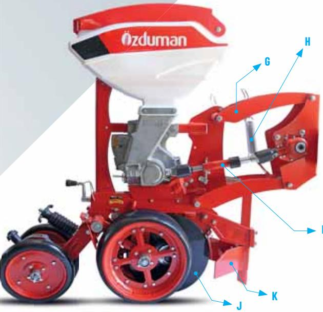
**A – Seed Tank :** 55-liter seed tank with a large volume is used for each seed variety.
